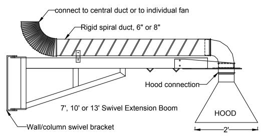
The series SB is constructed from heavy 2" x 2" and 4" x 2" heavy wall tube. All steel tubing is powder coated industrial grade epoxy paint for longevity.
