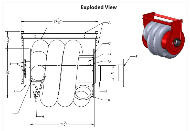
NOTE: The above dimensions are the same for both the motor operated hose reel and the widened version of the spring retractable hose reel (Series 9000-W).
