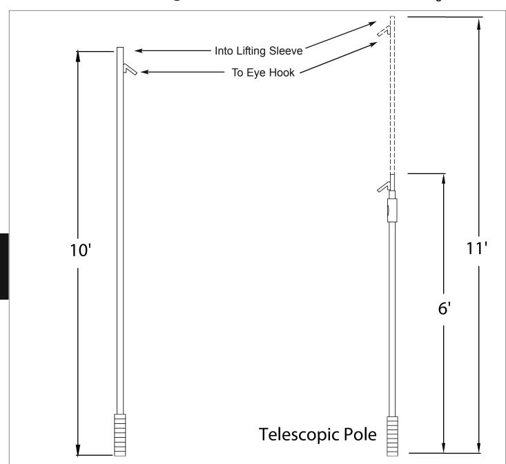
NOTE: An optional hook can be attached to the lifting pole. A vertical stack adapter will have a mating eye for the hook. This is commonly used when the adapter is on a hose reel or system with the balancer where the adapter may need to be pulled down from the overhead storage position.
