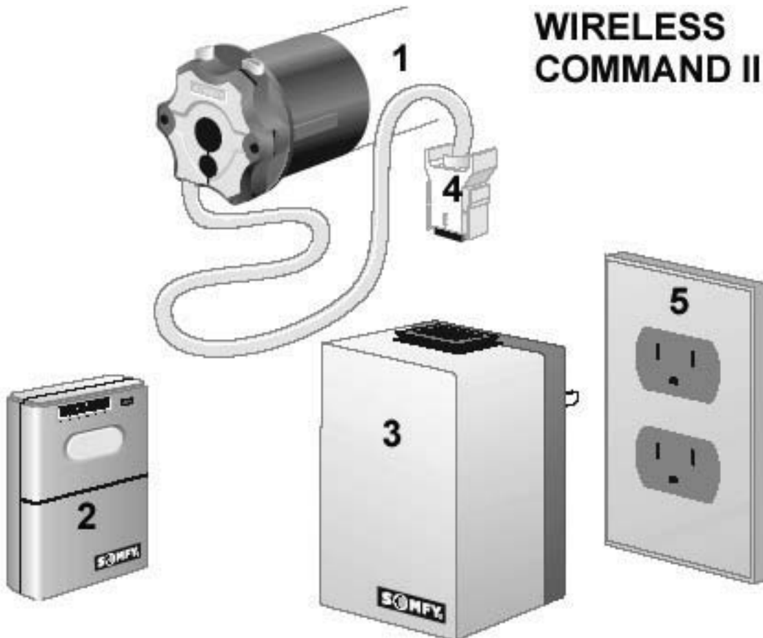
1-Direct Drive Motor Supplied on the Hose Reel; 2-Transmitter; 3-Controller; 4-Pre-wired plug supplied on the direct drive motor; 5-120 VAC outlet supplied on the hose reel
