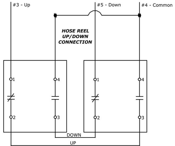
2-Button Pendulum for “up/down” control of motorized hose reel.
