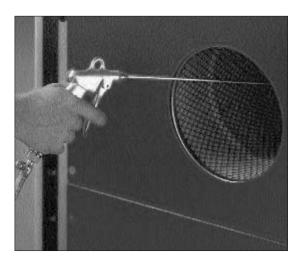
The PCFS is supplied with a unique manual air pulse filter cleaning system. Quick filter access is obtained through the hinged air plenum door, which exposes the inside of the cartridge filter. An air wand is then used and makes cleaning of the cartridge quick and clean. This manual cleaning procedure eliminates electric/pnuematic pulse valves and other components that can fail.
