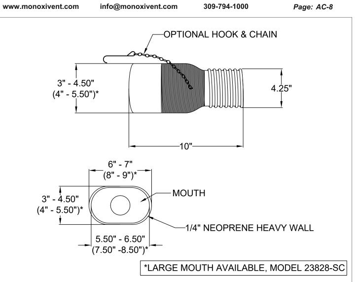
The oval body tailpipe adapter is constructed of 600-degree heavy wall neoprene rubber. The connection end has convolutions to screw into the mating hose. Adapters are also supplied with a connection sleeve to allow the adapter to attach to all Monoxivent hose: 1000, 2000, 3000, 4000, and 5000.
