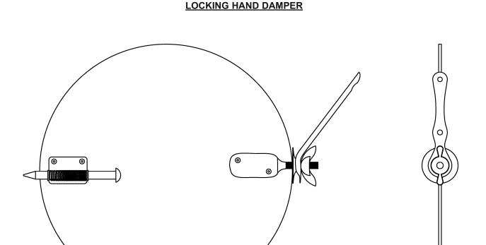
Locking hand dampers may be used for many applications. The dampers may be used on vehicle exhaust adapters and nozzles, welding cone nozzles, hard duct, or may be spliced into fabric duct.
