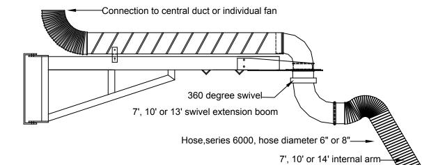
The Swivel Boom extension is constructed from 2" x 2" and 4" x 2" Heavy Steel Tube. The boom is powder coated with industrial grade epoxy combination for longevity. The arm offers complete vertical positioning movement and will swivel 180 degrees when wall mounted (additional travel is possible when column mounted) at the point of connection of the elbow to the boom end. The extension boom also pivots freely at the wall/column bracket.
