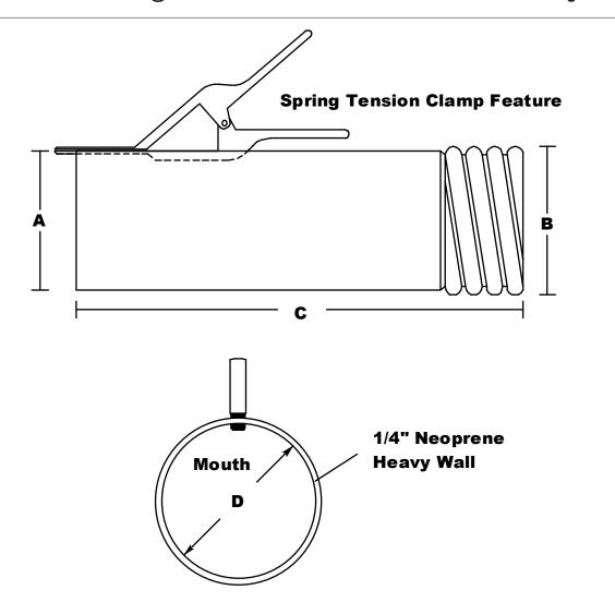
The Monoxivent clamping tailpipe adapter is constructed of 600-degree neoprene rubber. The adapter is supplied with a spring tension clamping device. The spring clamp is attached to the adapter body, allowing a positive connection to the vehicle tailpipe. A simple squeeze on the spring clamp handles allows quick attachment to the tailpipe. The adapter can be removed by another simple squeeze or a direct pull on the adapter or hose. The clamping adapter can be used on all series hose.
