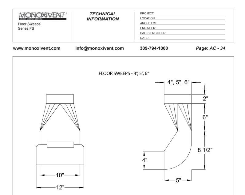
Floor sweeps are manufactured from 20-gauge galvanized steel for strength and rigidity. A continuous piano hinge connects the door to the fitting. Available in 4", 5", or 6" models. Other sizes - fabrication available, please consult factory.
