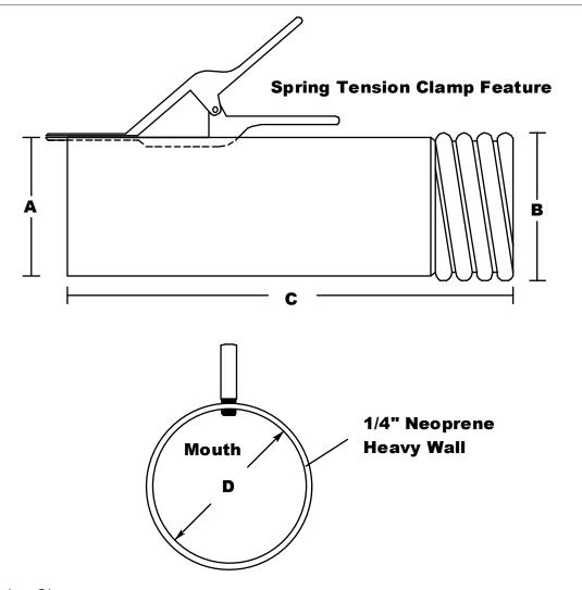
Hose Connection Sizes 23897-SC - 4" or 5" No Crush Hose 23897-SC-SL - 4", 5", or 6" Fabric Hose
