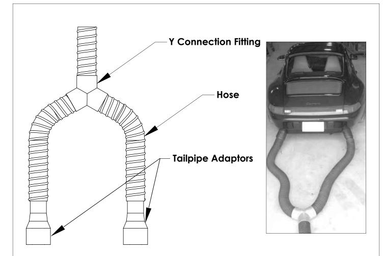
NOTE: The Y Kit Assembly is available for various configurations. Please specify your applications and the factory will set-up the required hose lengths, distances, and adapters. Y Kits are offered in 3", 4", 5", and 6" diameters. Hose can be made of "no crush" hose (shown above) or fabric type. Y fitting will be supplied to fit the standard tailpipe adapter, so the assembly can be easily removed or the Y assembly can be permanently fixed to the extraction hose.
