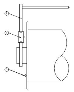
Switch Assembly Mounted To Hose Reel
