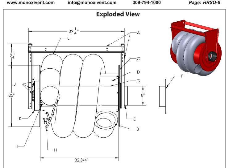
NOTE: The above dimensions are the same for both the motor operated hose reel and the widened version of the spring retractable hose reel (Series 9000-W).
