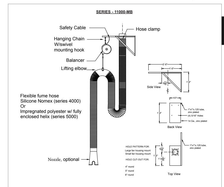
**NOTE:** 11000-MB System is supplied with a Mounting Bracket (as shown)
