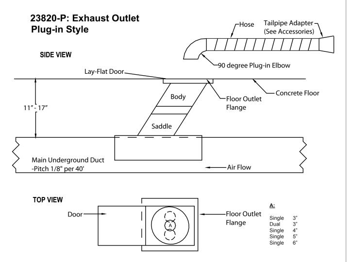
Lay-flat door is opened, exposing the inner plate that will have one of the combinations denoted by "A" in the top view (above). The hose/plug-in elbow is inserted into the "A" opening, which completes the connection from the floor outlet to the vehicle. (Hose, typically, is stored on a wall structure or column within the building.)
