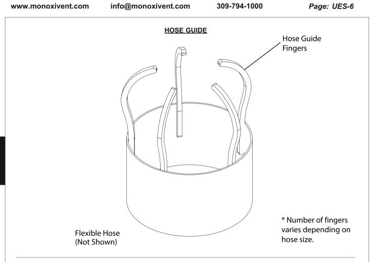
The Hose Guide is used to assist the hose used for the underground system. The Hose Guide is attached to the end of the hose. The Hose Guide assists the hose during its return into the main underground duct.
