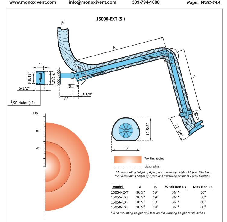
Nozzle: Injection molded in with hood plate in anodized aluminum.
