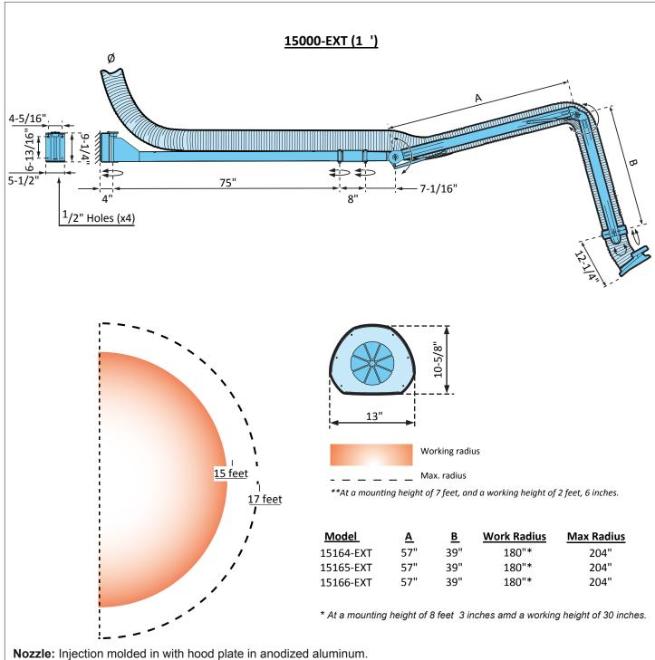
**Nozzle:** Injection molded in with hood plate in anodized aluminum. **Hose:** Hose of dark-blue PE-coated polyamide fabric rated to 215 degrees F. Other options available (chemical & abrasion resistant) - please consult factory Optional light kit or fan/damper switch available.
